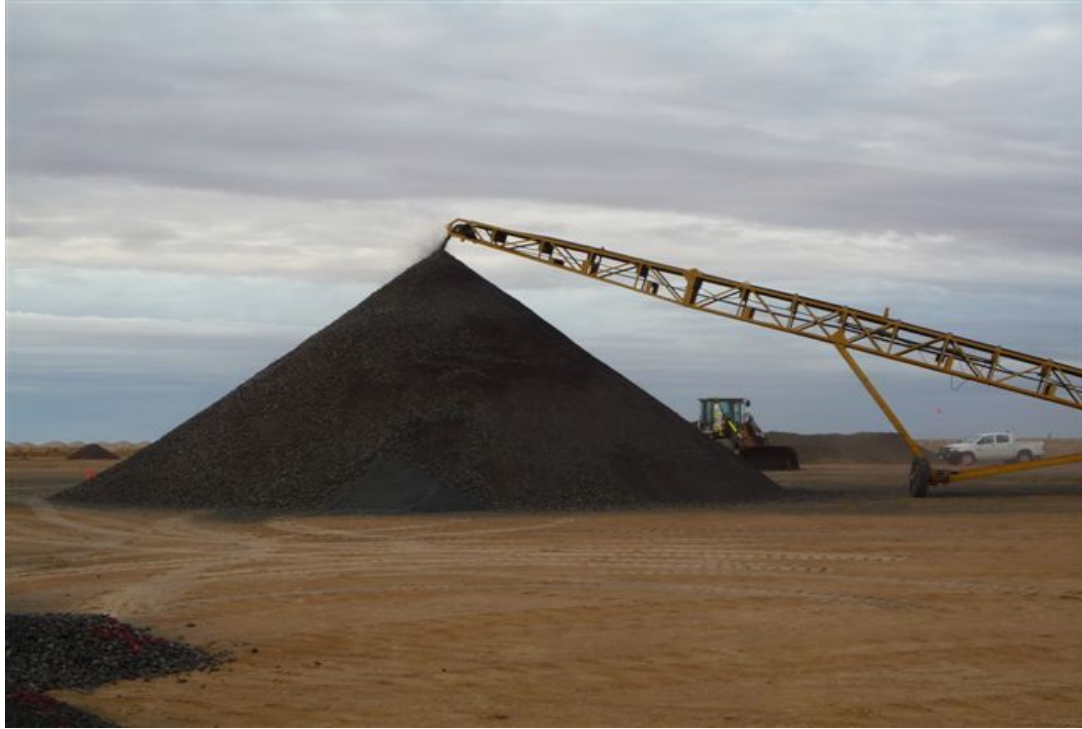
Figure 2: Crusher Stacker and Crushed Ore Stockpile.
